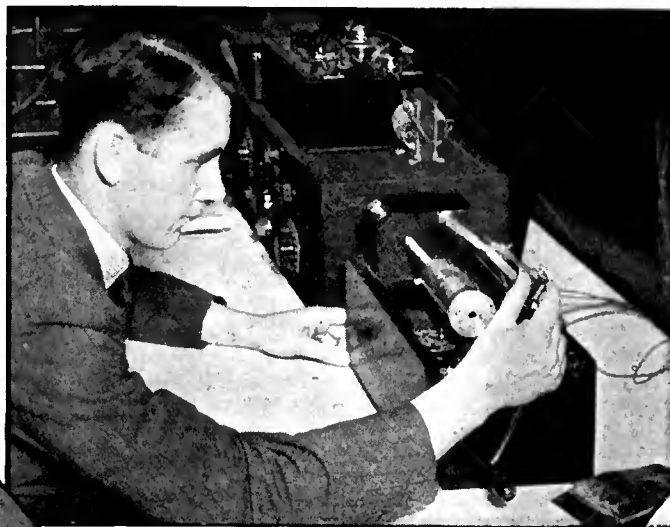
These pictures show the Fultograph apparatus which is used by the British Broadcasting Company for the broadcasting of pictures. (above) The apparatus being set in motion at Station 2LO, (left) adjusting the paper to the receiving cylinder, and (right) a cartoon as it is received on the cylinder
